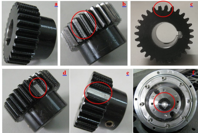
Figure 2. Pictures of the measured sun gear. a-normal, b-surface wear, c-crack, d-chipped, e-tooth missing, f-the measured sun gear
